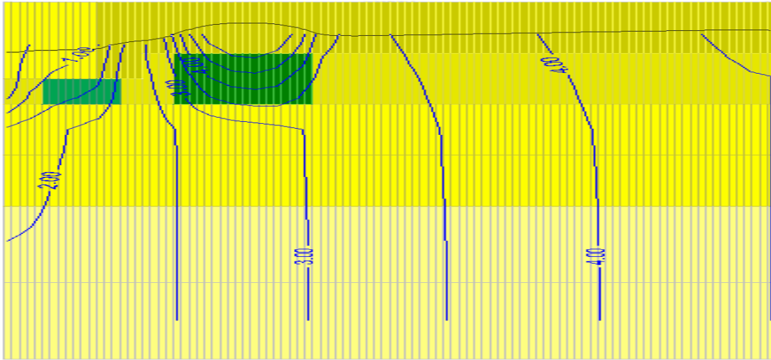
Model Diagram 1 (vertical scale exaggerated) Simulated Hydraulic Heads Shown in Cross-Sectional View (Green zones represent clay layers. Yellow zones represent sand and gravel units; lighter colors indicate higher hydraulic conductivities)
