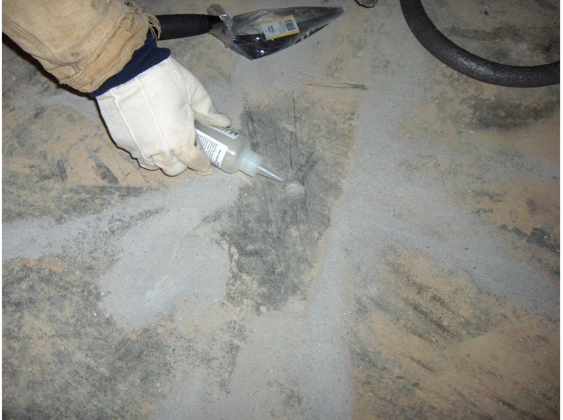
Photo 1, Smoke test at test point
