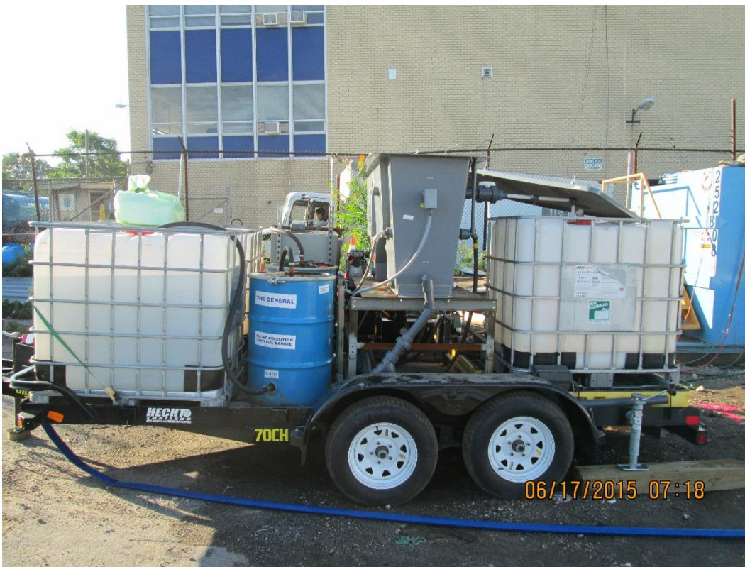
Oil water separator running on RAD II
