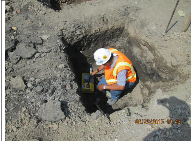
Compaction test on pier footings for equipment trailers
