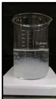
Beaker #2 Formation of the PersulfOx Catalyst in PersulfOx and water solution post addition of 10% wt/wt solution of \text{H}_2\text{SO}_4 resulting in pH 7
