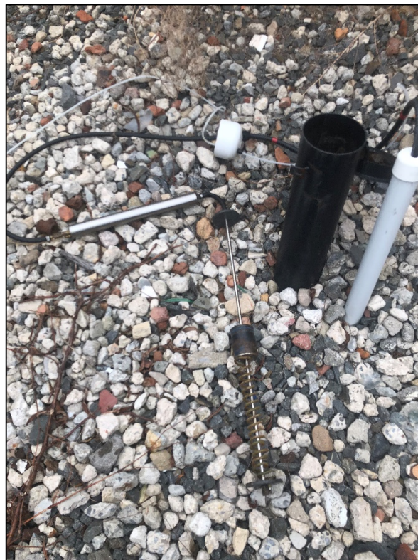
Photograph 14: One of five Geotech AC Sipper pumps installed in recovery wells
