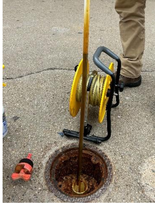
Product observed coating and mixed within bailer from C241175 MW-37S .
