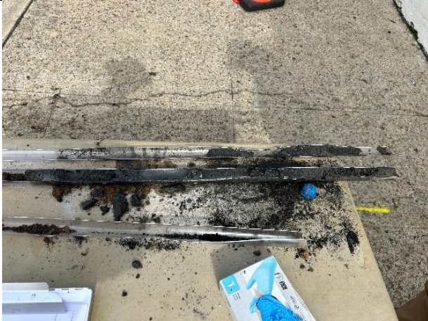
Soil profile from SB-5 (10-15 ft bg) with stained soil visible
