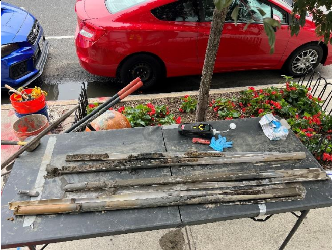
Soil profile from OS-SB-9 (5-20) with staining, odor, and 308 ppm at groundwater interface (~7-8')
