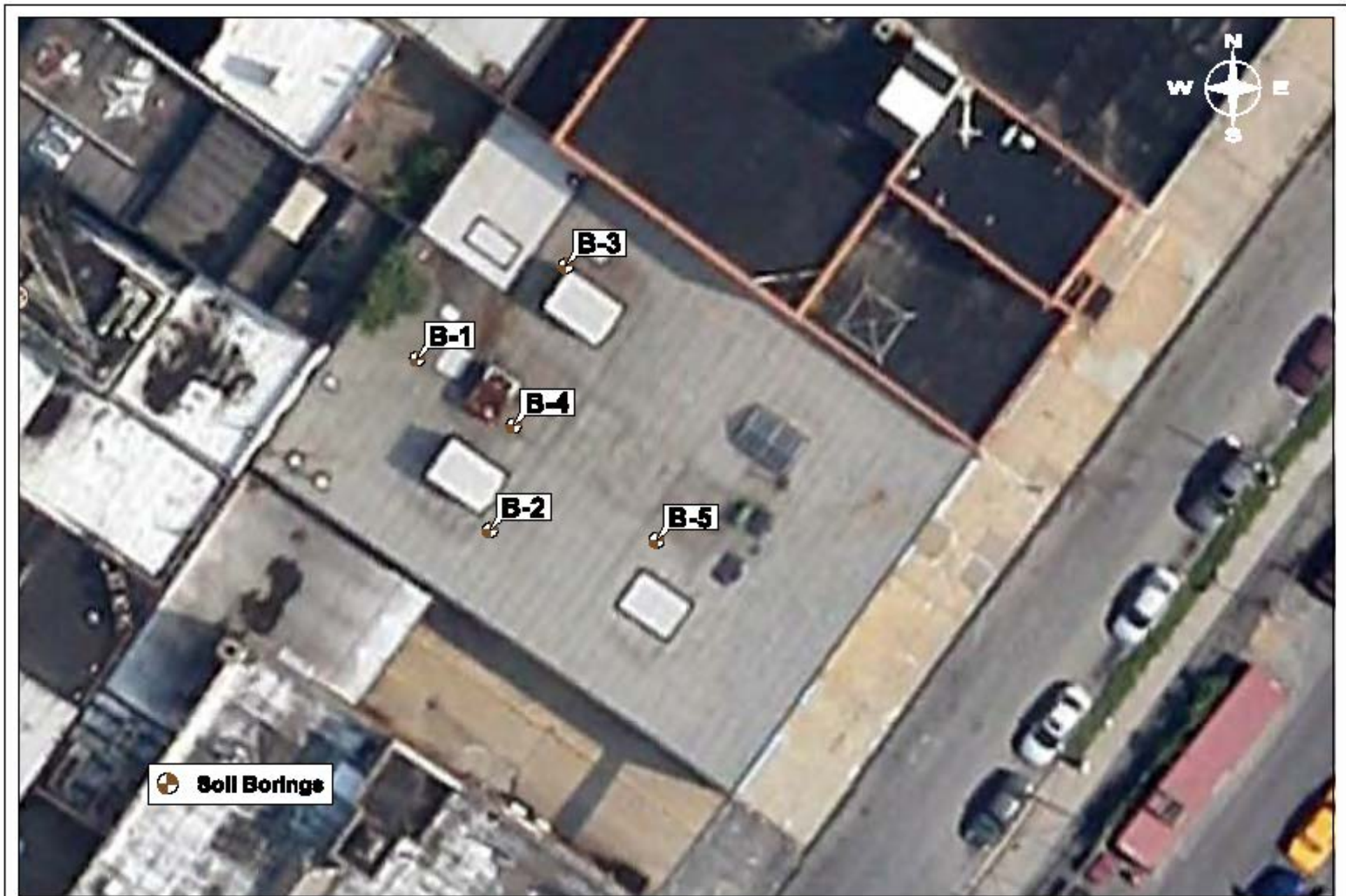
Figure 4 Soil Boring and Soil Sample Locations
