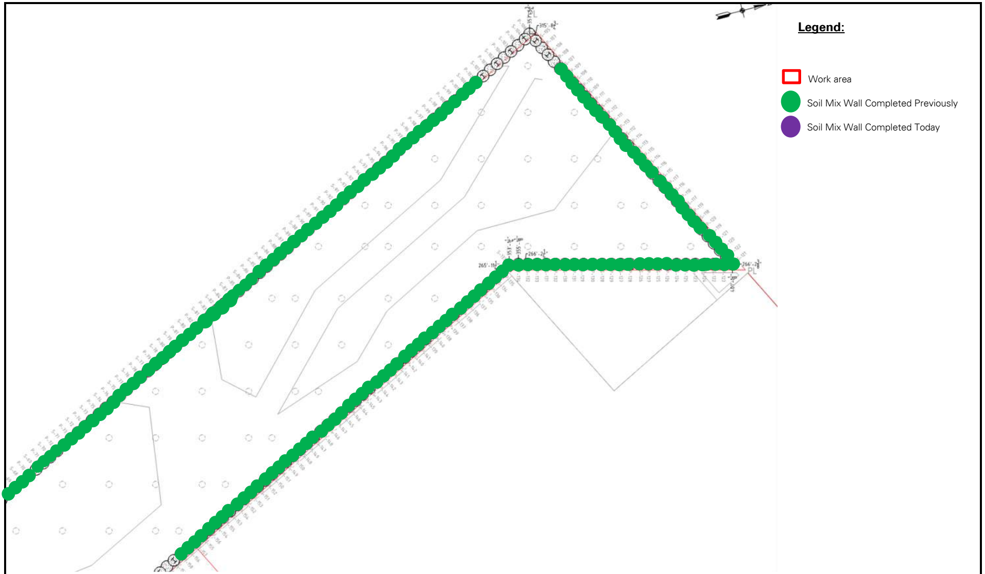
Figure 2A – Soil Mix Wall (taken from drawing: SOE coordinate part plan 1, dated 06/09/2025)
