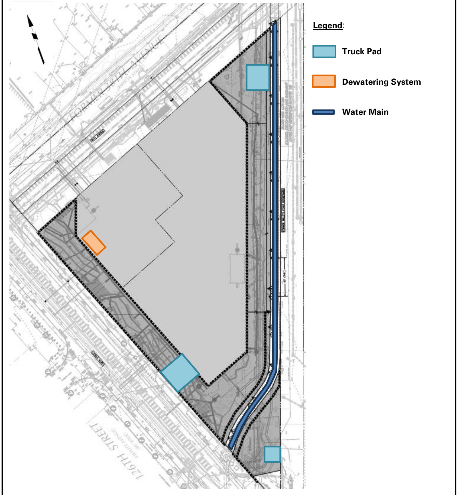
FIGURE 1: Support of Excavation Plan, Site Features
