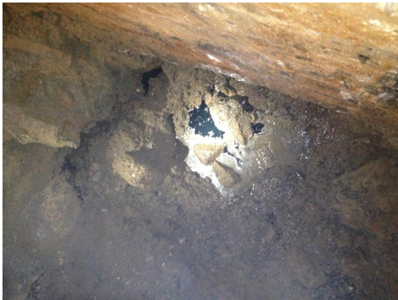
Photograph 2: View of the grossly contaminated soil and LNAPL identified in the geotechnical test pit.
