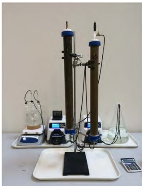
Figure 9. O -Xylene column study set-up
