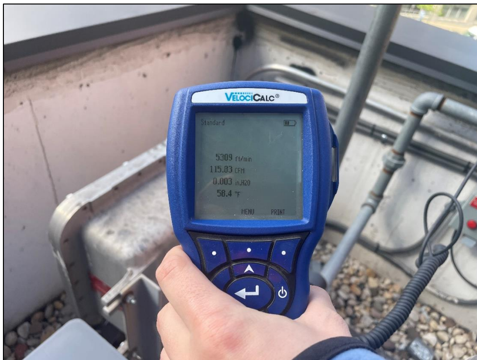
Photo 6, 05/17/2023: View of flow readings collected from the south blower (facing southwest).
