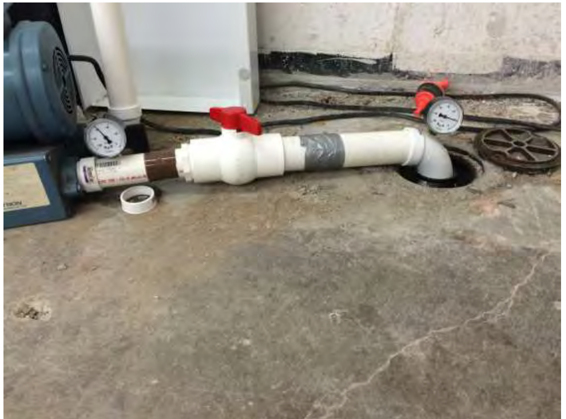
Test 2 – Throttle at 45 degrees, Pressure Readings
