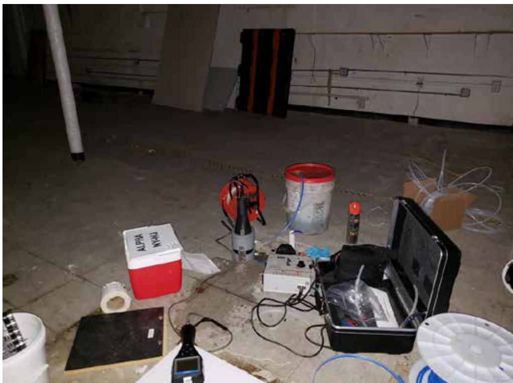
Photo 11: Low flow sampling of MW3.
