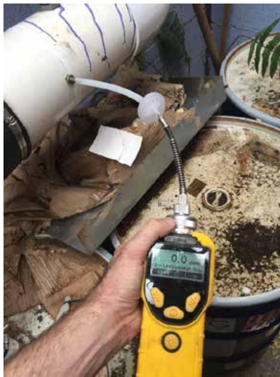
Photo 4: Post-carbon sampling point showing 0.0 ppm.
