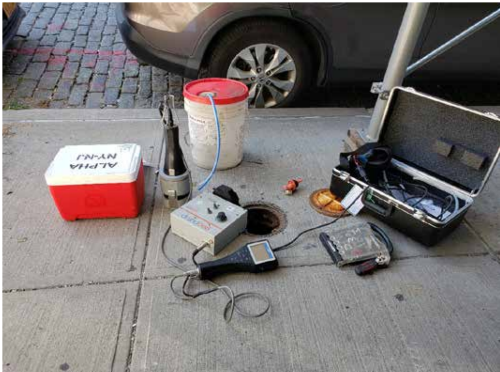
Photo 10: Low flow sampling of MW3 ADJ.
