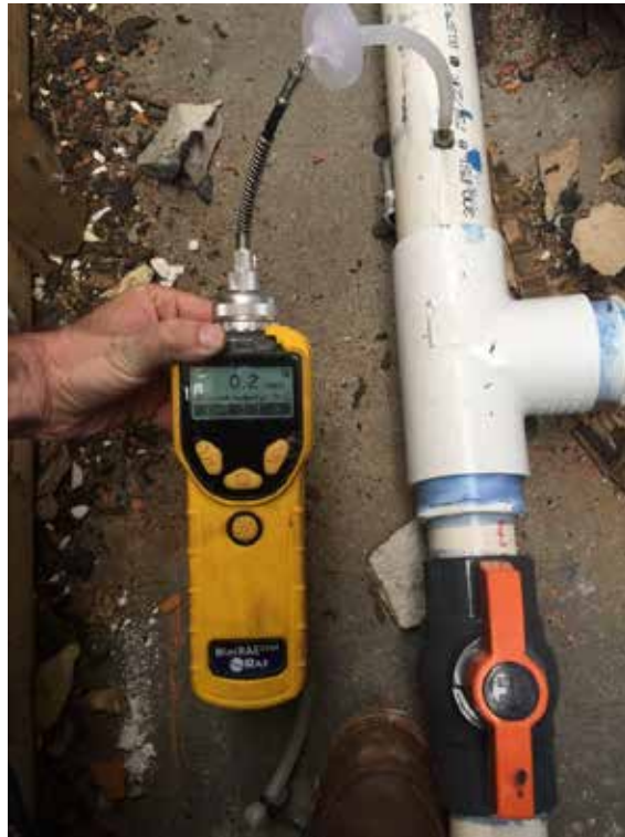
Photo 3: Pre-carbon sampling point showing 0.2 ppm.
