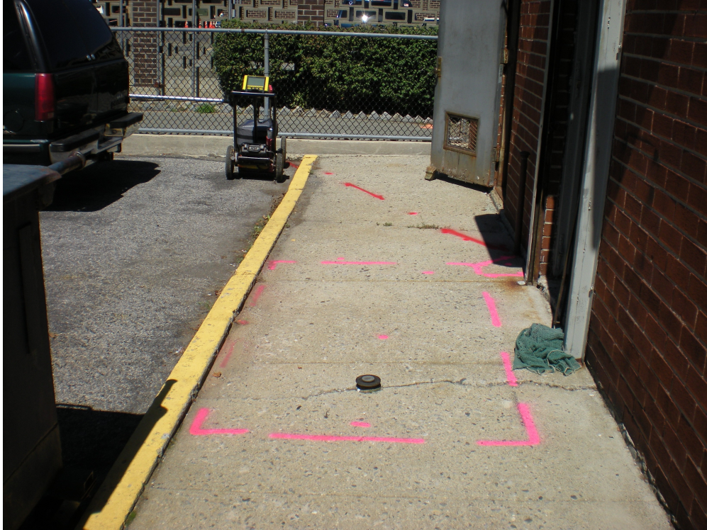
Figure 1 – Metallic anomaly consistent with an UST and associated piping designated with pink paint. Note the electrical line nearby designated in red.
