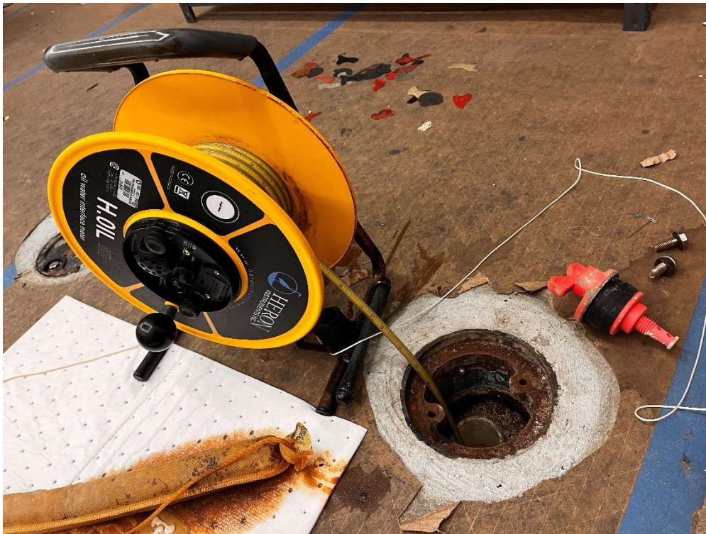
Photo 8 (2/17/2024): View of Langan gauging LNAPL at MW34D
