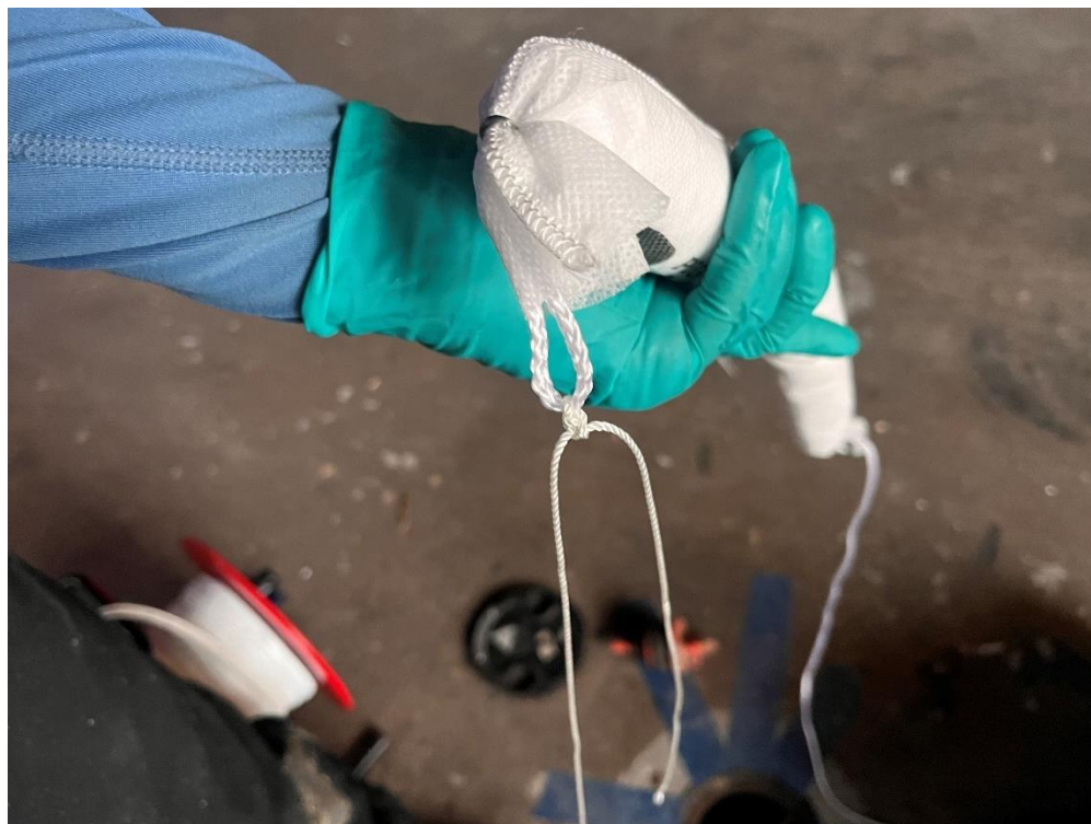
Photo 3 (2/10/2024): View of Langan installing an absorbent sock at MW30D
