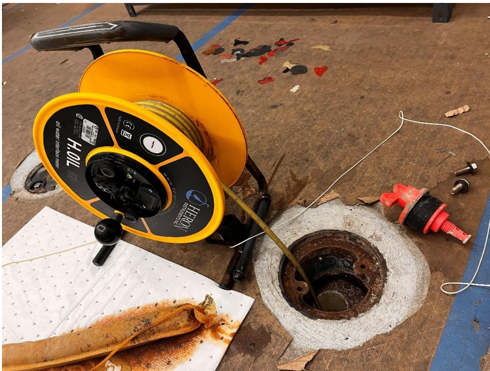
Photo 8 (2/17/2024): View of Langan gauging LNAPL at MW34D
