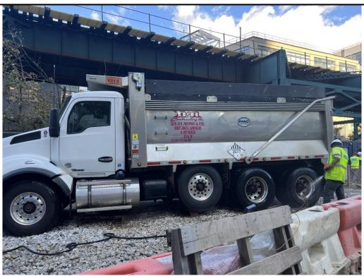
Photo 3: A truck with a built-in tarp preparing to leave site (facing west).
