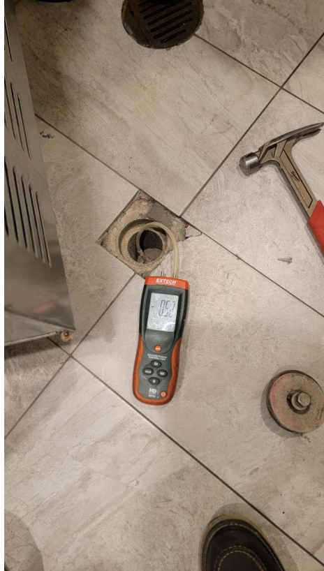
9- Sub-slab vacuum monitoring in cellar
