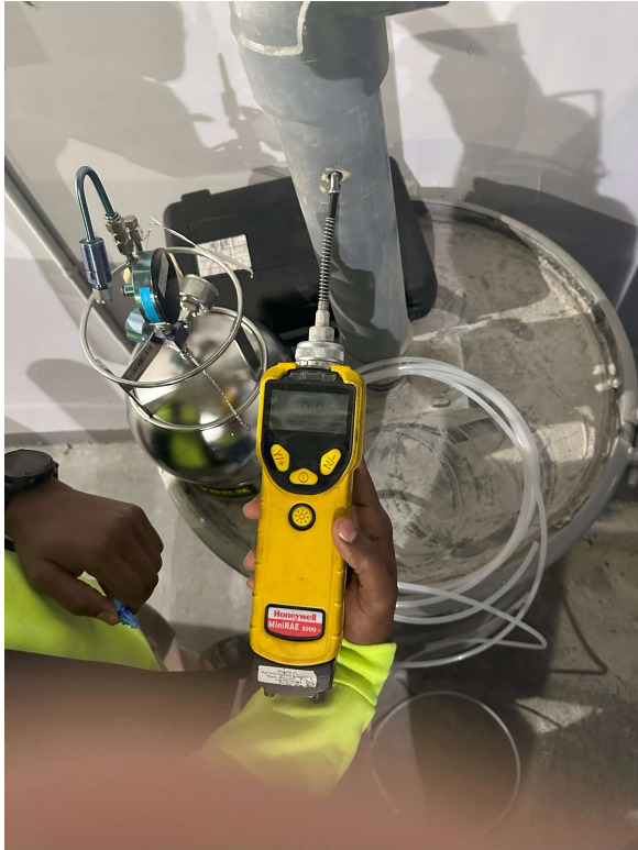
11-View of effluent monitoring of organic vapors/air flow and GAC sampling
