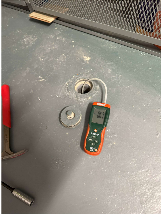
10- Sub-slab vacuum monitoring in sub-cellar
