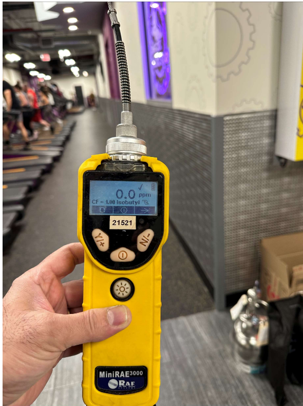
1- Organic vapor assessment in indoor air with PID
