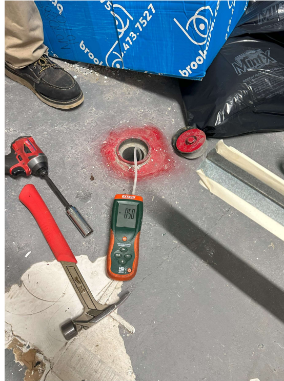
10- Sub-slab vacuum monitoring in sub-cellar
