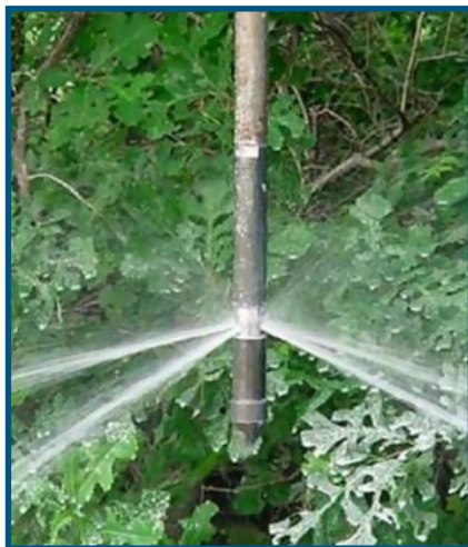
FIGURE 6 Image of Geoprobe® pressure activated injection probe
