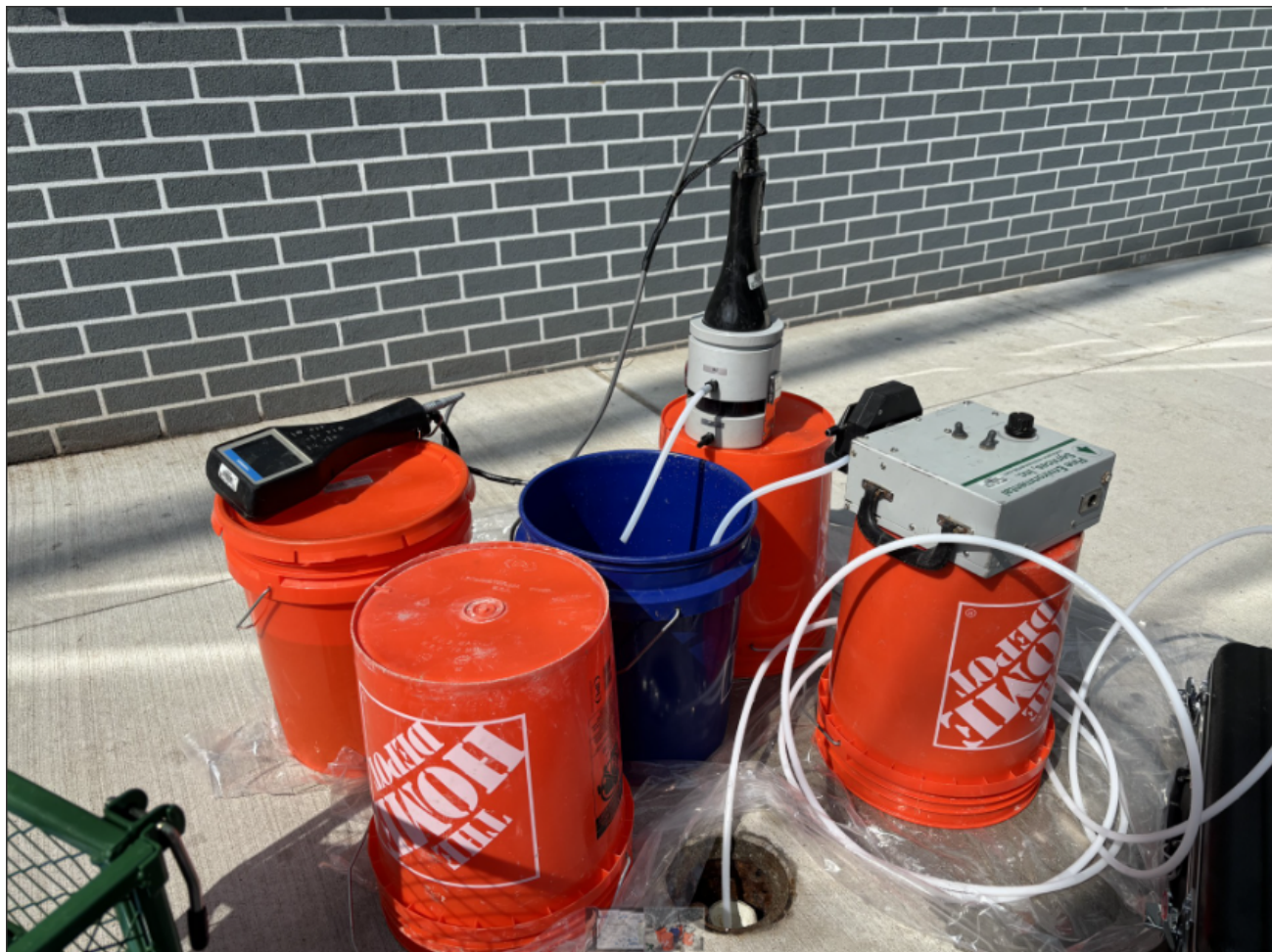
Photo 2: Low-Flow Groundwater Sampling at Monitoring Well MW-5.
