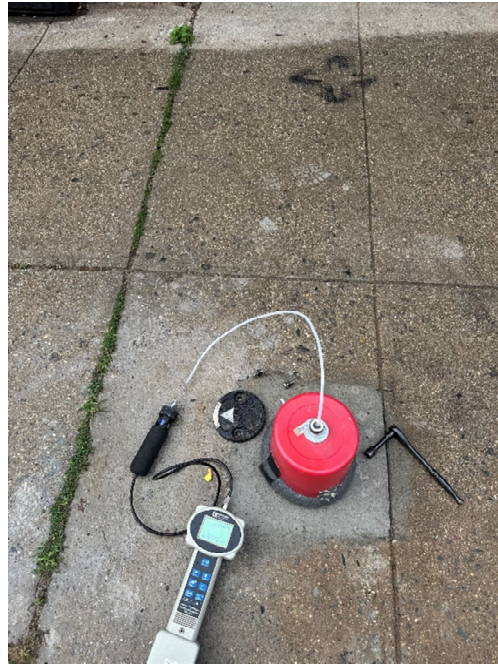
Photo 4: Bucket test being set up
