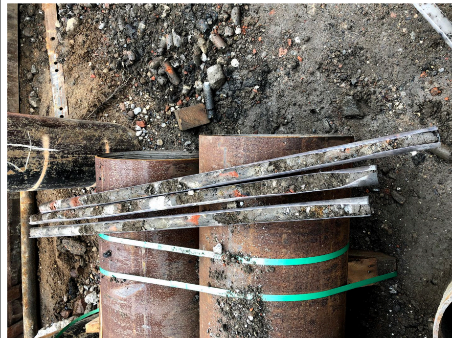
Photo 2: View of soil borings from WCG-3C (0-7').
