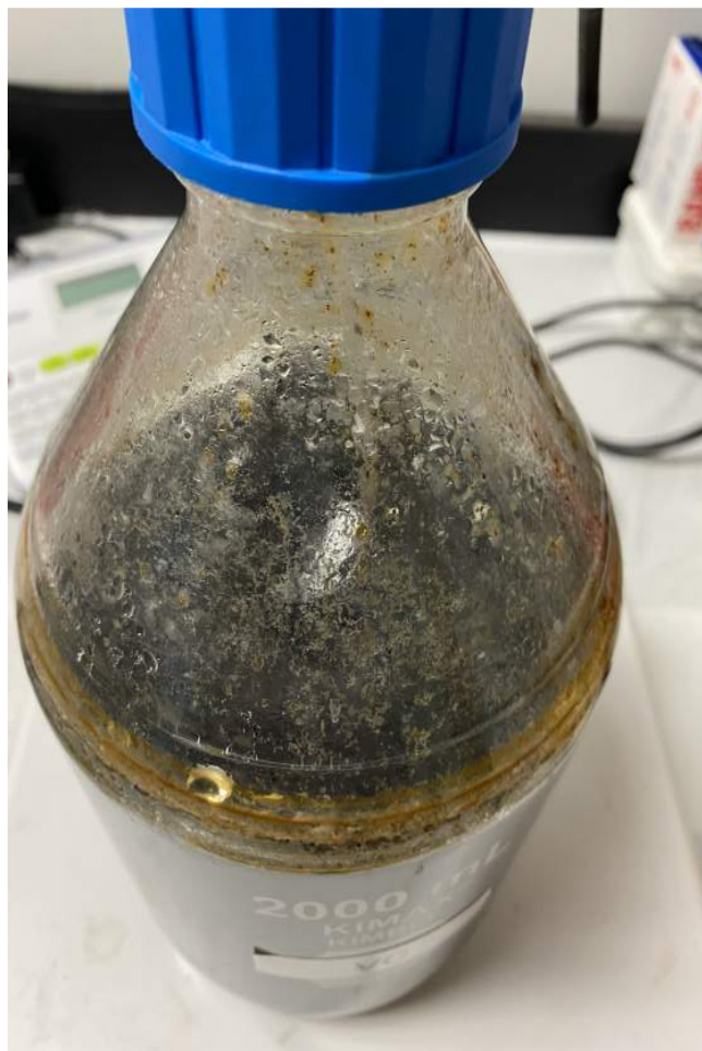
Photo 16: Rusty material visible in treated VC jar (Week 2)
