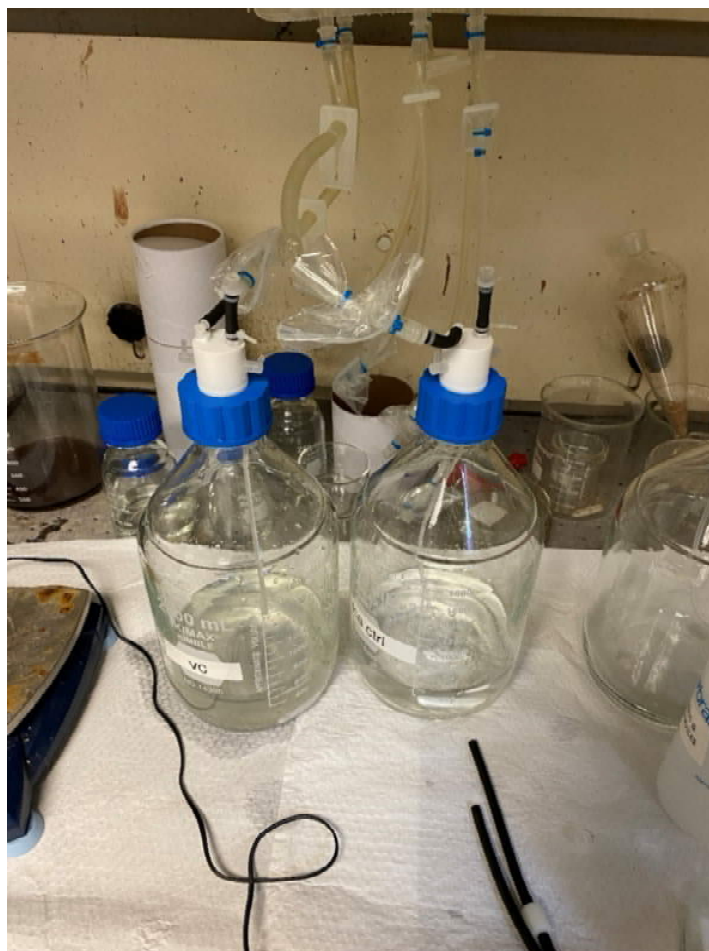
Photo 1: Filling 2 L jars with groundwater from Labtainer bags (treatability study setup).
