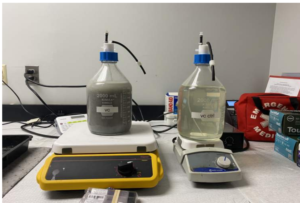
Photo 8: VC jars filled to 2 L mark on stir plates (treatability study setup).
