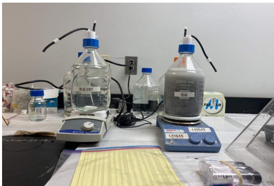
Photo 7: TCA jars filled to 2 L mark on stir plates (treatability study setup).
