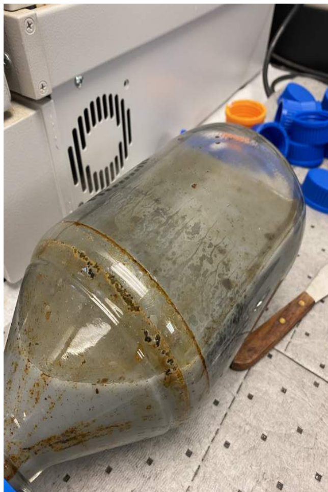
Photo 17: Rusty material visible in treated TCA jar (Week 2)
