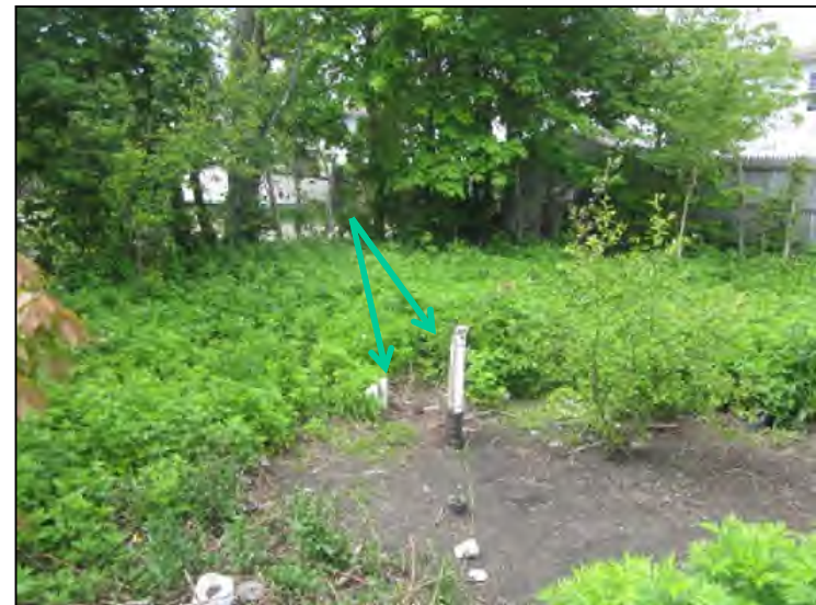
Photograph 4. A grassy patch in the southwestern corner of the Property, with monitoring wells for a permeable pavement pilot test.
