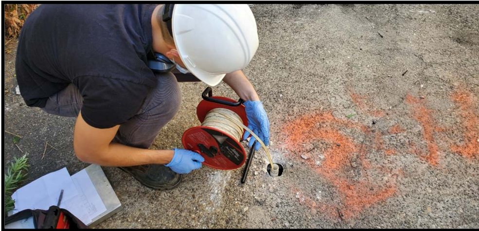
View of a monitoring well being gauged prior to sampling.
