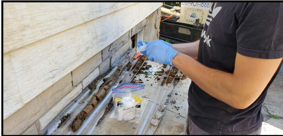
View of a soil sample being collected from a soil boring.
