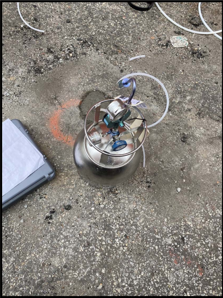
View of a soil vapor point being sampled.
