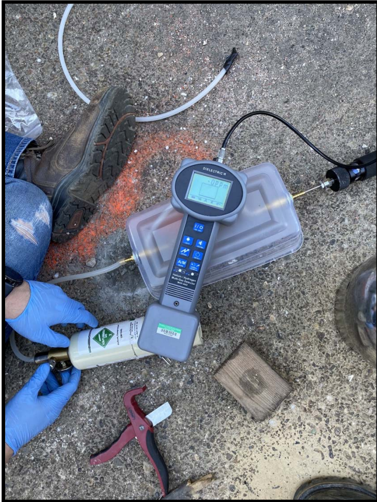
View of a soil vapor sampling point being leak checked prior to sampling.
