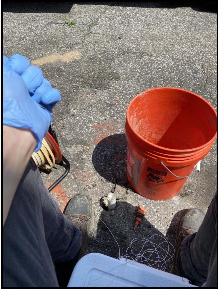
View of a monitoring well being purged prior to sampling.
