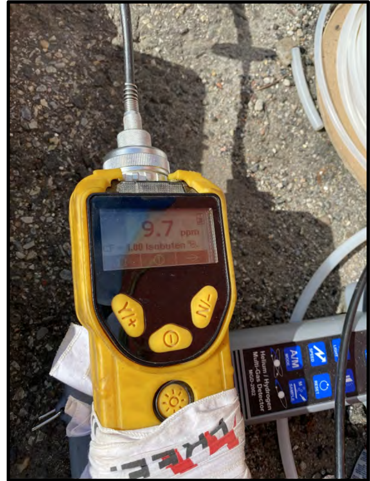
View of a soil vapor sampling point being purged prior to sampling.
