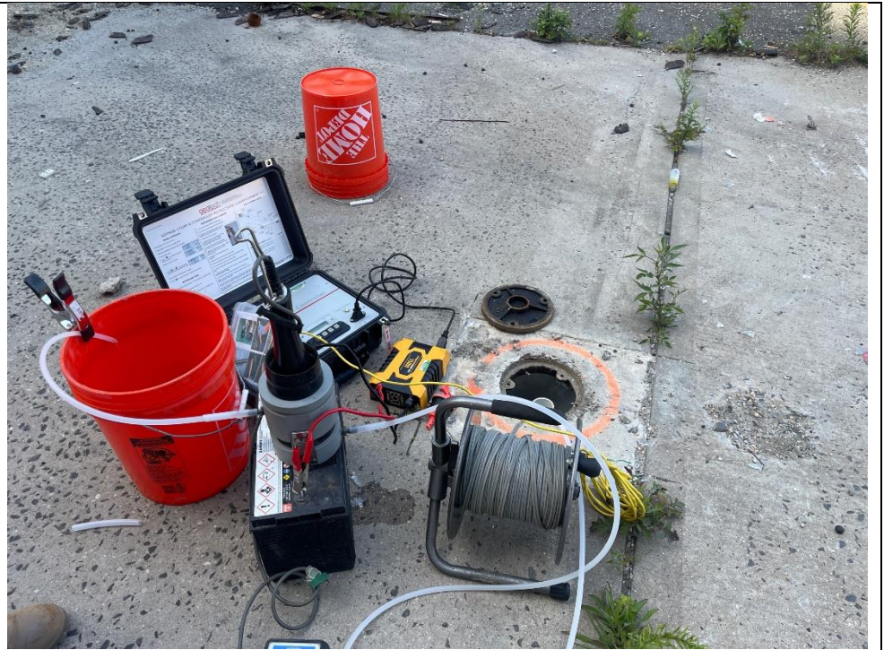
Photo 3 – Photo of typical low flow groundwater sampling apparatus and setup
