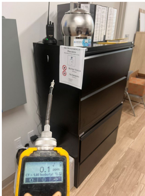
Photograph No. 15: View of ambient PID readings collected from the interior of the building.
