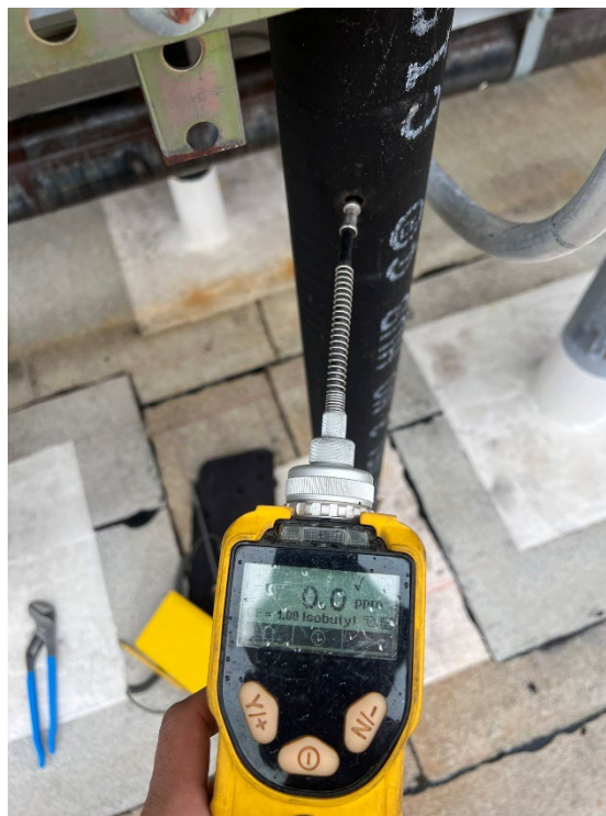
Photograph No. 16. View of PID readings collected from risers located in the roof area.
