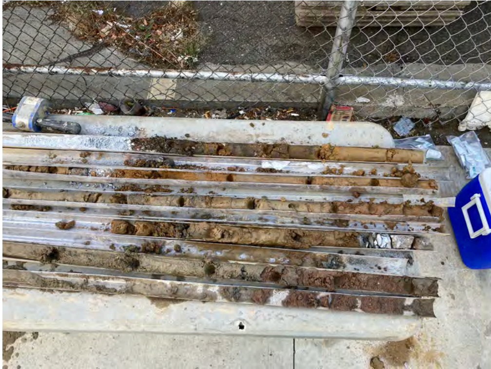
Photo 13: Soil boring material collected from TRC-SB-23 from 0 to 25 feet below ground surface (bgs), typical.
