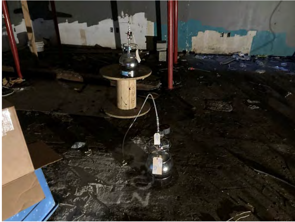
Photo 7: Collection of sub-slab soil vapor sample, TRC-SSV-03 and co-located indoor air sample, TRC-IA-03.
