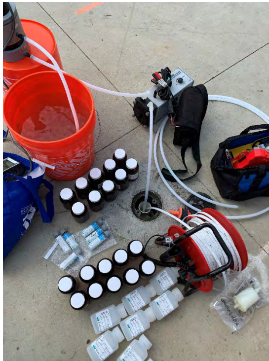
Photo 10: Groundwater sampling set up at monitoring well, TRC-MW-29, typical.
