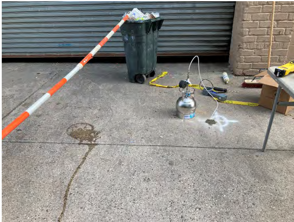
Photo 6: Collection of soil vapor sample, TRC-SV-09, on sidewalk of Queens Street.
