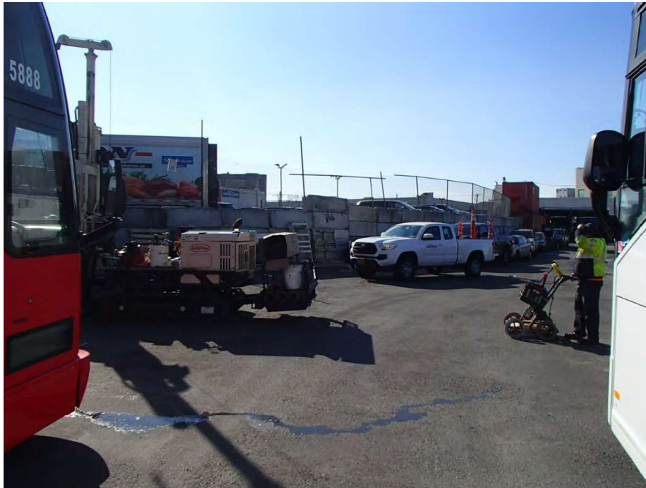
Photograph 3: View of the ground penetrating radar (GPR) equipment utilized to identify subsurface anomalies.
