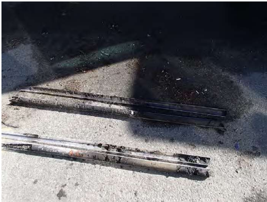
Photograph 6: View of a soil core the exhibits the presence of historic fill material and organic material.
