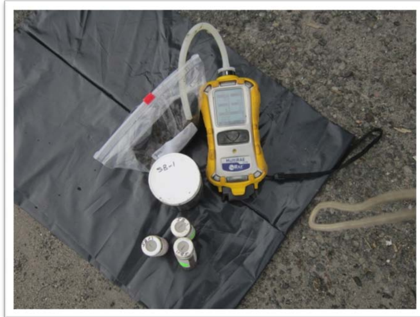
5. A Typical PID Reading by Utilizing MultiRAE
