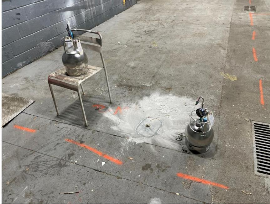
**Photo 1:** Sample collection at sub-slab soil vapor sample SSV-2 and indoor air sample IA-2 (facing east)
