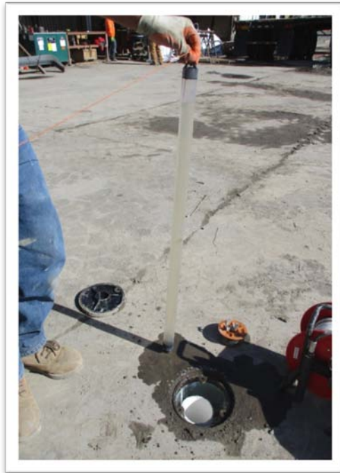
10. GW Sampling from MW-1 by Utilizing Bailer
