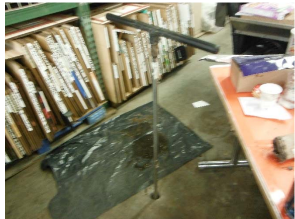
Photograph Nos. 9 & 10: In addition to the air samples collected, one (1) soil sample was collected from the northwest portion of the building. The soil sample was collected from a soil boring installed utilizing a manually operated stainless steel hand auger, in a location where a two-inch diameter coring drill borehole was installed through the concrete slab prior to Preferred's Soil Vapor Intrusion Study, by others.
