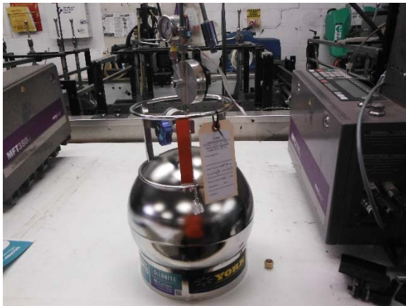
Photograph No. 8: One (1) indoor air sample was also collected, proximate to the SSV sample location within the northern portion of the building. Both the indoor air sample and the SSV sample were collected with 6-liter Summa canisters utilizing a 24-hour regulator.
