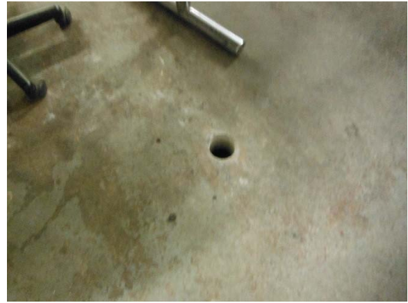
Photograph Nos. 9 & 10: In addition to the air samples collected, one (1) soil sample was collected from the northwest portion of the building. The soil sample was collected from a soil boring installed utilizing a manually operated stainless steel hand auger, in a location where a two-inch diameter coring drill borehole was installed through the concrete slab prior to Preferred's Soil Vapor Intrusion Study, by others.
