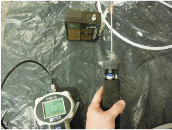
Photographs No. 7: A required helium test was performed (with a helium detector, pictured above) to ensure the integrity of the sampling procedures.
