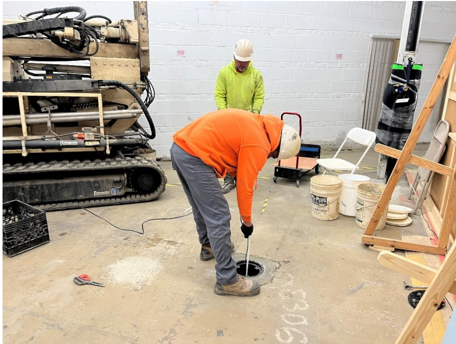
Photo 1: Placing the submersible pump and tubing in monitoring well MW-6 for well development.
