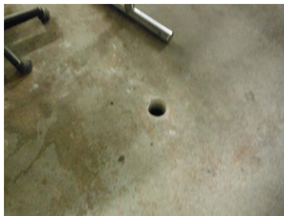
Photograph Nos. 9 & 10: In addition to the air samples collected, one (1) soil sample was collected from the northwest portion of the building. The soil sample was collected from a soil boring installed utilizing a manually operated stainless steel hand auger, in a location where a two-inch diameter coring drill borehole was installed through the concrete slab prior to Preferred's Soil Vapor Intrusion Study, by others.
