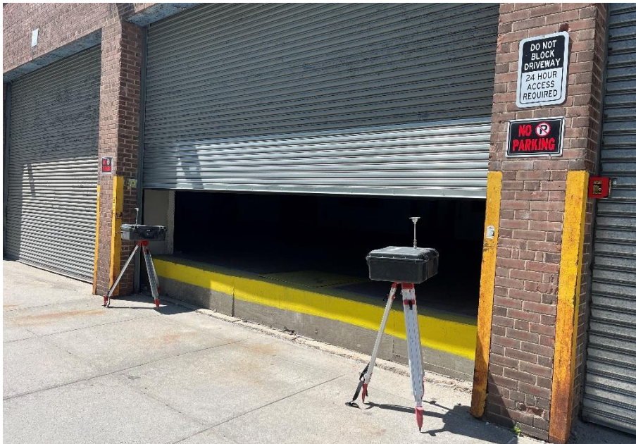
Photo 2: CAMP monitoring along 30 th Street at bay door nearest work area to SB11.
