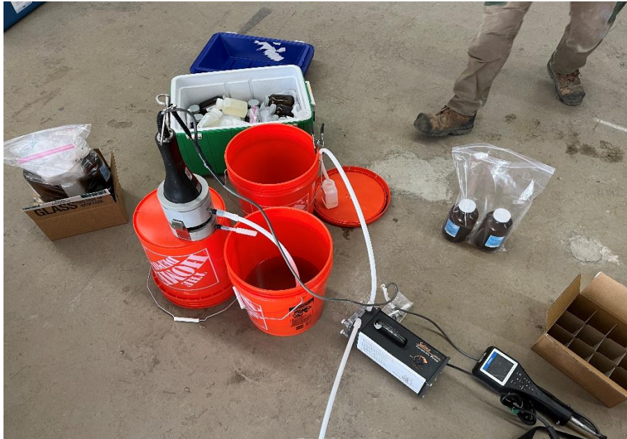
Photo 1: Langan sampling groundwater from groundwater monitoring well MW-5
