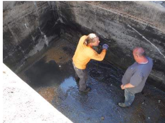
Photograph No. 12 - Field screening of soils underlying the concrete vault noted the presence of fill material absent of diesel odors and elevated PID responses.
