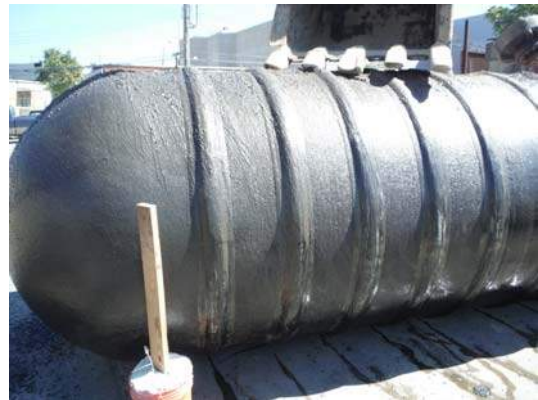
Photograph Nos. 5 & 6- Inspection of the 4,000-gallon single-wall fiberglass UST noted the absence of any holes or cracks that did not appear to be sustained during the removal efforts.
