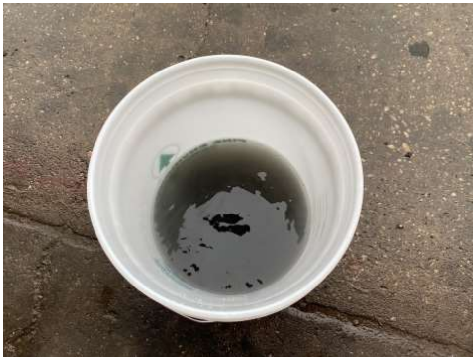
Photograph 5: View of purged groundwater generated from development of temporary monitoring well MW02
