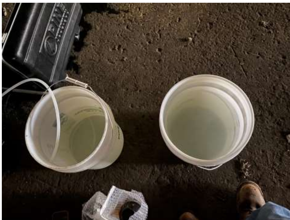
Photograph 6: View of purged groundwater generated during low flow purging of temporary monitoring well MW02, prior to groundwater sample collection.
