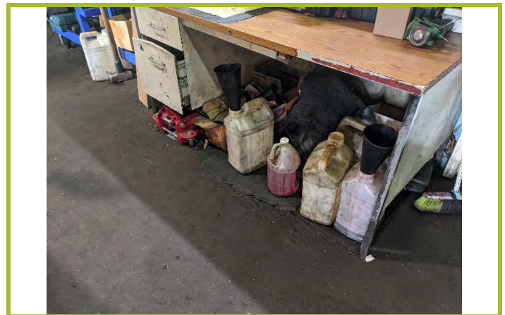
Photo #6: Typical unlabeled containers of automotive fluids in Maintenance Garage.
