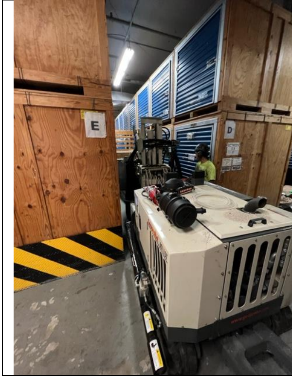
Soil Probe Installation at Subject Property
