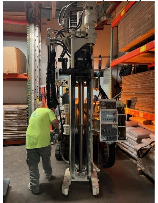
Soil Probe Installation at Subject Property
