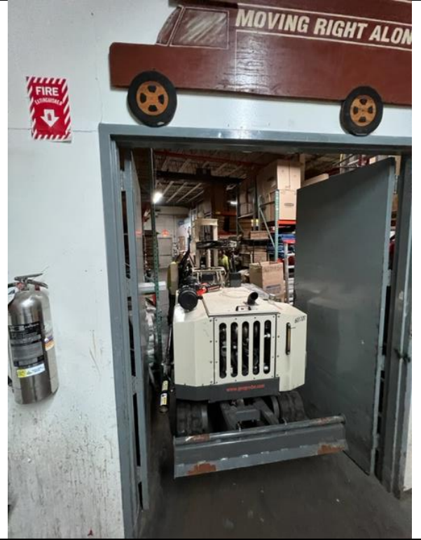
Soil Probe Installation at Subject Property
