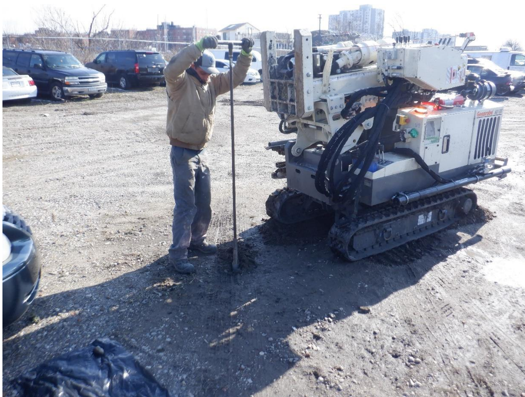
Photograph No. 1 & 2: View of drill technician hand-clearing sampling locations prior to utilization of a remote access rig to complete soil borings on the subject property located at Beach 62nd St, Queens, NY.
