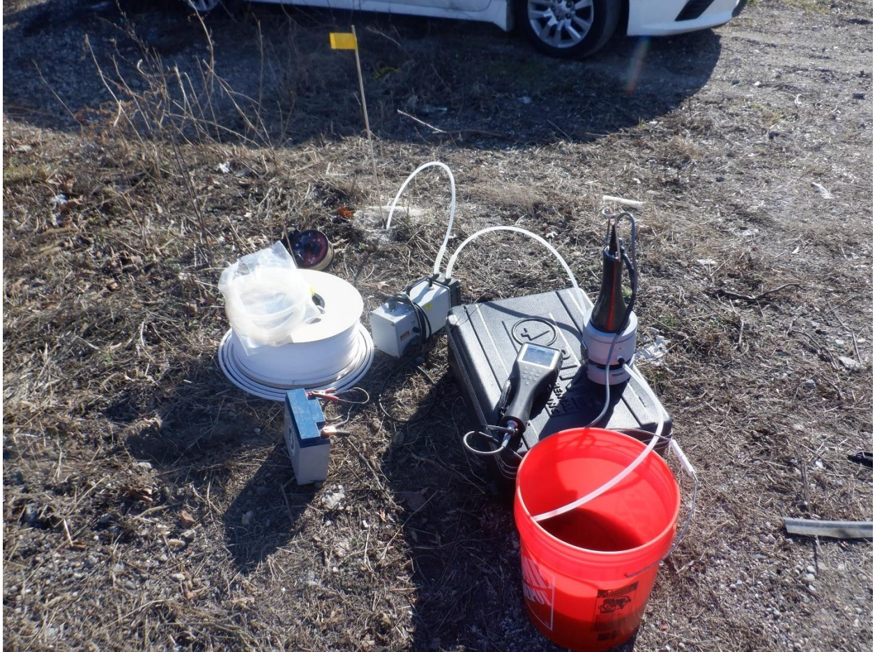
Photograph No. 7: Groundwater samples were procured from the three (3) temporary groundwater monitoring wells installed on the subject property. Field parameters were collected via utilization of a Horiba.
