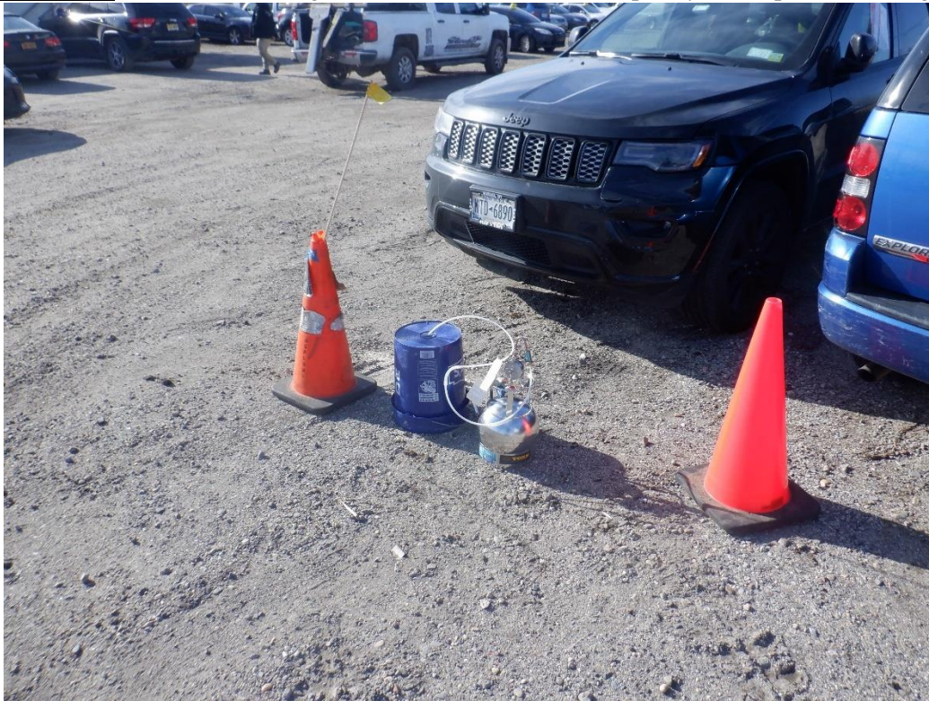
Photograph No. 4 & 5: Three (3) sub slab soil vapor samples and one (1) outdoor air sample were collected from the subject property during the investigation. Helium leak detection testing was performed on the soil gas and sub slab vapor samples prior to the collection of the air samples.
