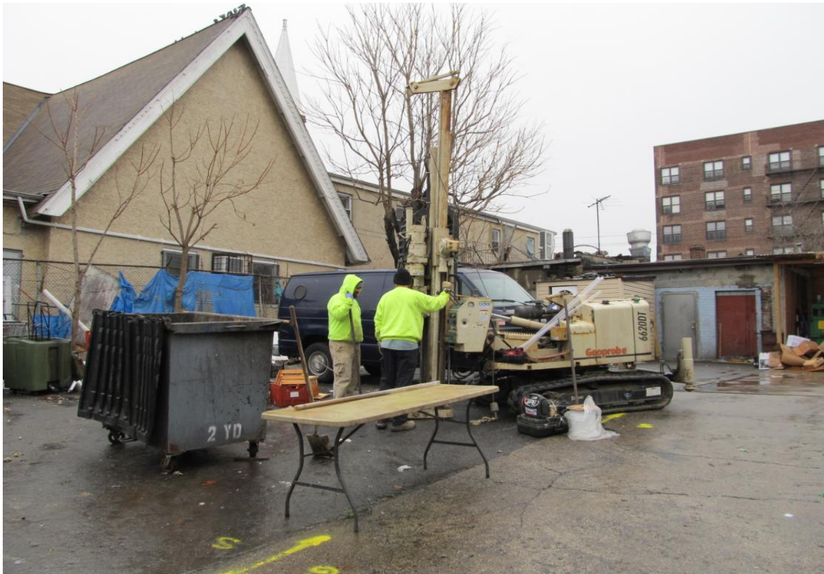
Figure 8: Completion of TB-3. No detectable concentrations of tetrachloroethylene were discovered in the soil or groundwater at this test location. Of note, the detectable contaminant concentrations increase closer to 1322 Central Avenue, the former cleaners location.
