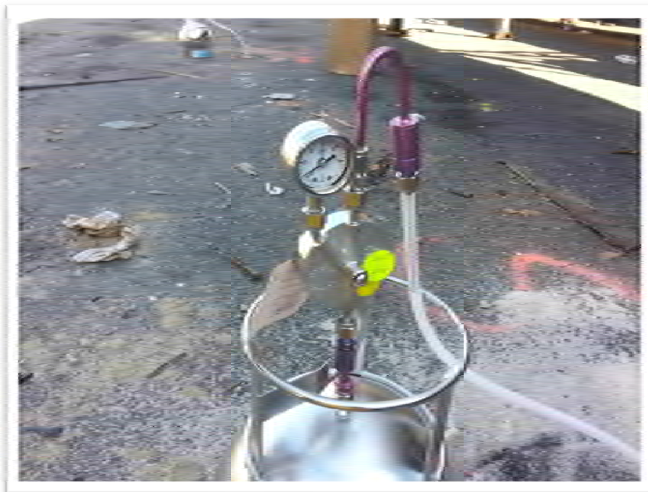
8. Typical Air Vapor Canister for Soil
