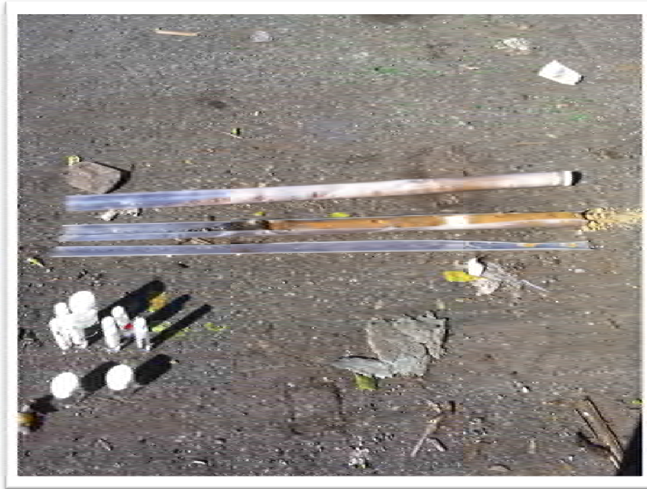
5. Soil Sleeves from the Soil Boring Four (SB-4)
