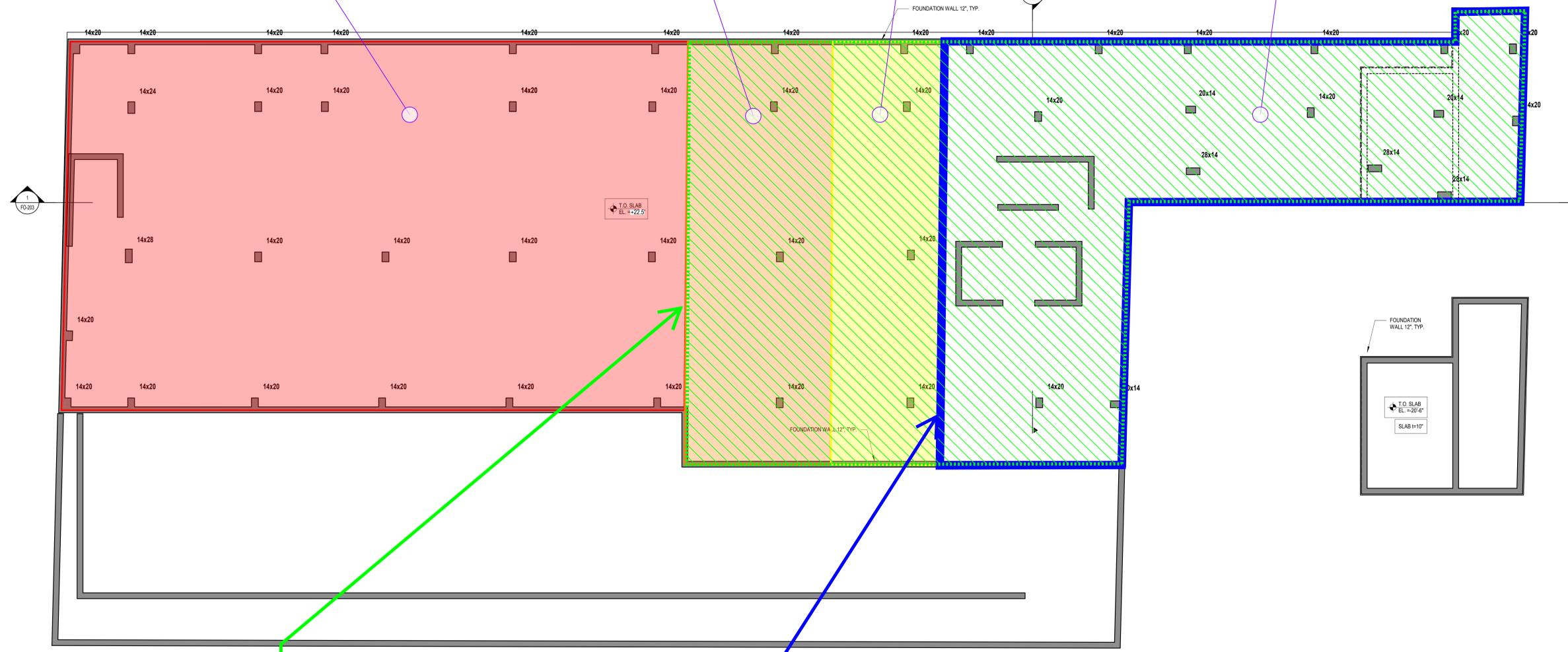
Approximate footprint (green hatching) where overexcavation below El. 21.5 to reach Stratum III Till (Class 3a) material will be required.
