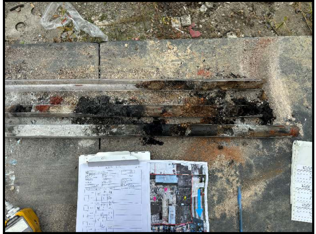
Typical view of soil boring being screened for VOCs by PID and geologically logged. SB-2 had an apparent petroleum impact odor and staining in the 0-2 feet interval.
