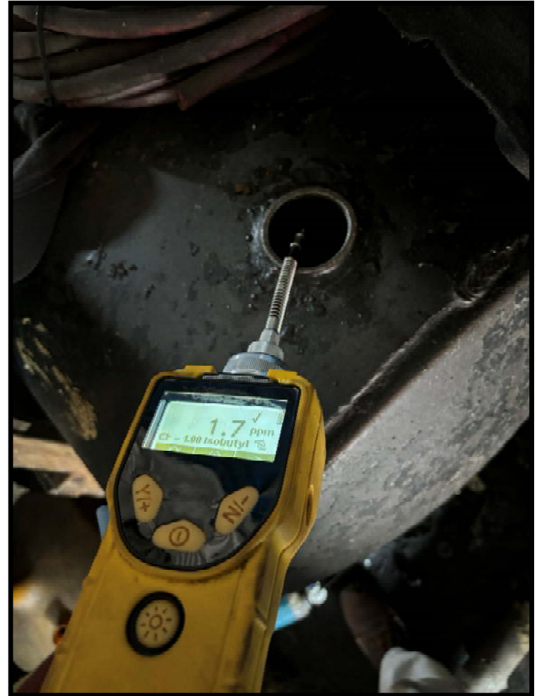
View of a PID reading of 1.7 ppm near a waste oil tank stored at an auto repair shop at the Site.
