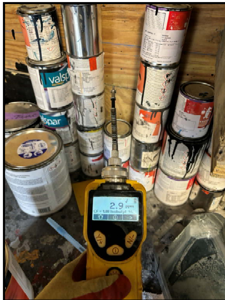
View of a PID reading of 2.9 ppm near paint containers stored at the auto body repair shop at the Site.
