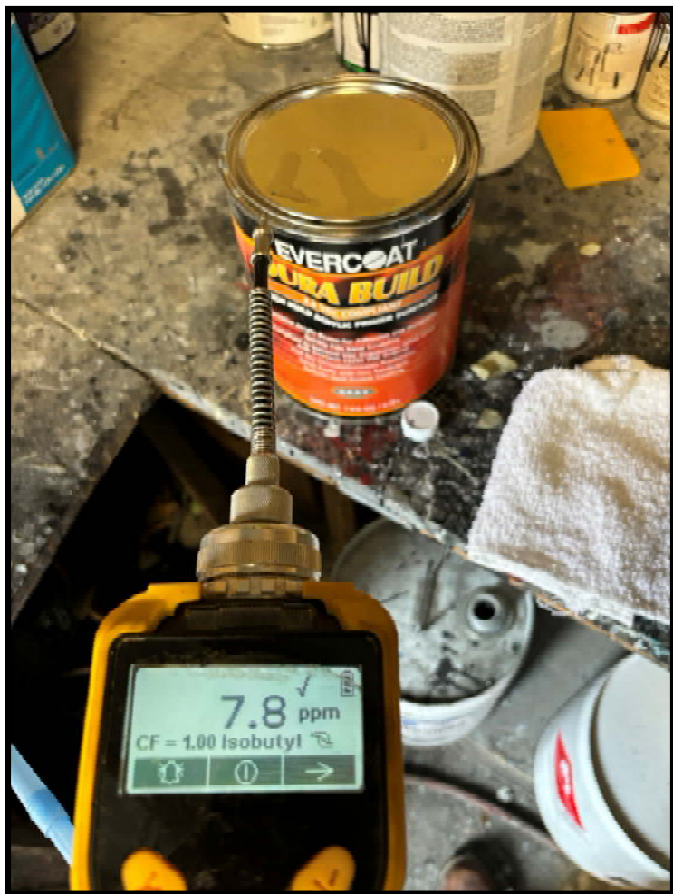
View of a PID reading of 7.8 ppm near an acrylic coating container stored at the auto body repair shop at the Site.
