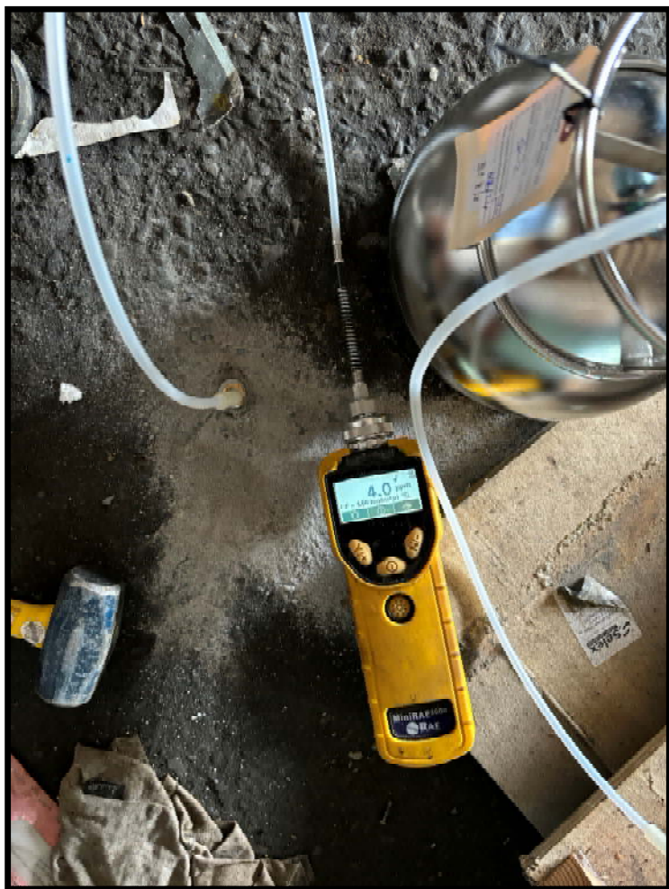
Typical view of a soil vapor point being purged with a PID, measuring 4.0 ppm.
