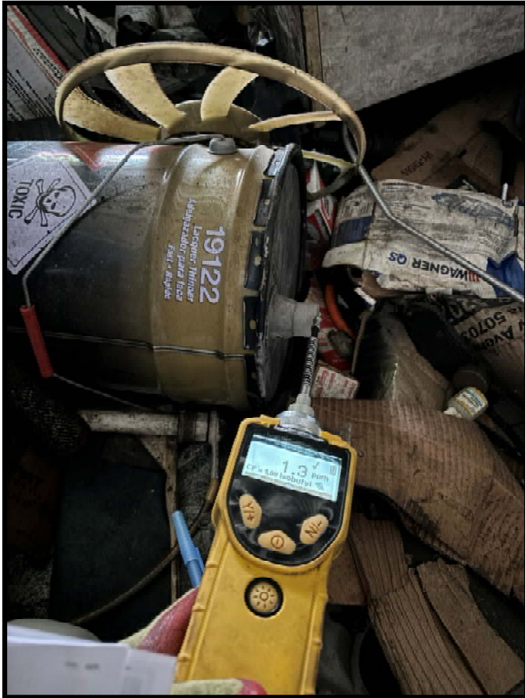
View of a PID reading of 1.3 ppm near a lacquer thinner container stored at one of the unoccupied Site buildings.
