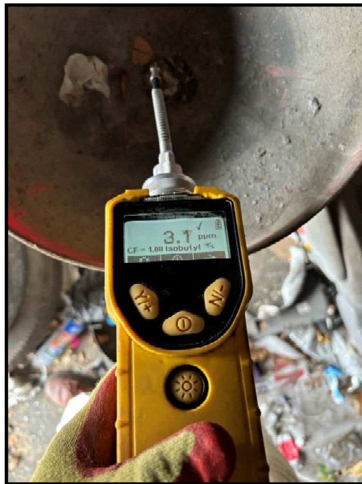
View of a PID reading of 3.1 ppm near a waste oil tank stored at one of the unoccupied Site buildings.
