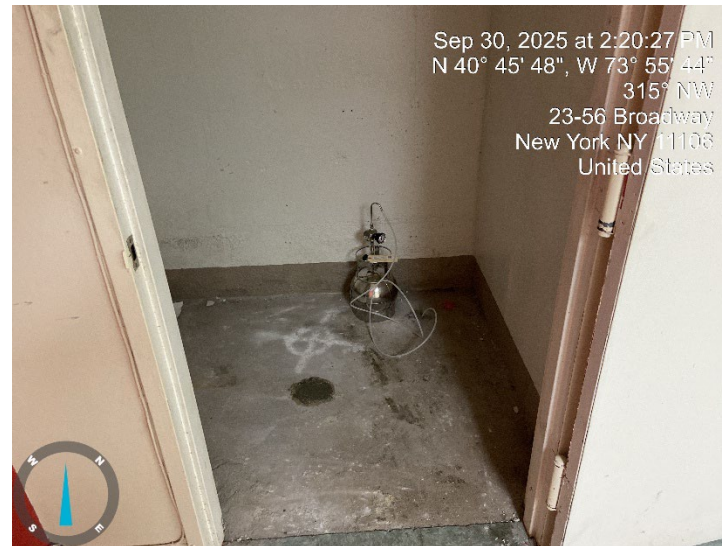
Photograph 4: View of soil vapor testing within the Site building.
